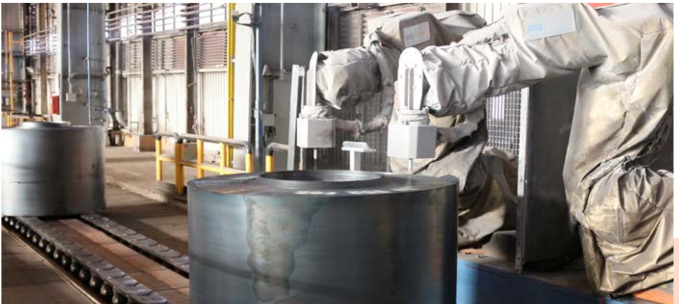
Two collaborative robots can share the markings, or one or both can make the full markings
